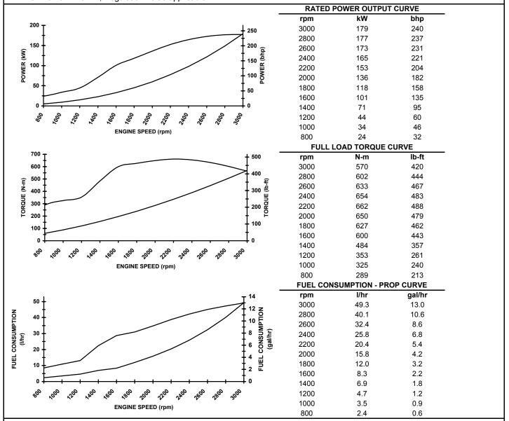
Rated Conditions: Ratings are based upon ISO 8665 and SAE J1228 reference conditions; air pressure of 100 kPa [29.612 in Hg], air temperature 25 °C [77°F], and 30% relative humidy. Power is in accordance with IMCI procedure. Member NMMA.
