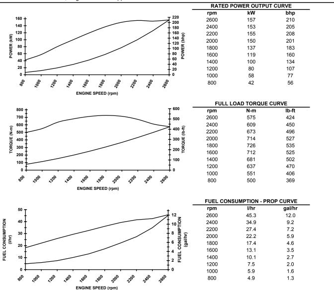
Rated Conditions: Ratings are based upon ISO 8665 and SAE J1228 reference conditions; air pressure of 100 kPa [29.612 in Hg], air temperature 25 °C [77°F], and 30% relative humidy. Power is in accordance with IMCI procedure. Member NMMA.
